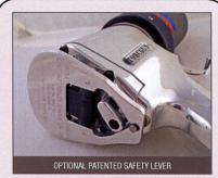
This safety mechanism drastically reduces operator error. The lever must be depressed while pulling the trigger, ensuring operator keeps hands away from pinch points.
